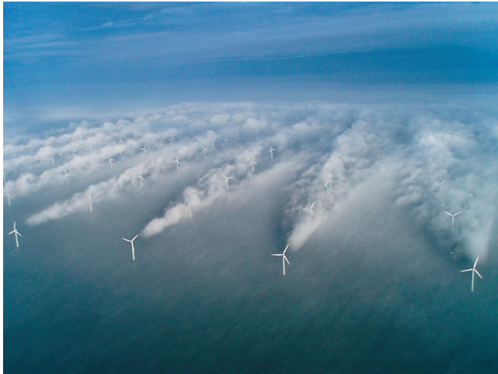
Figure: Cloud formation in a wind farm in high humidity air. The turbulence behind the turbines leads to the nucleation of water droplets. The condensation releases the large latent heat of the vapor to fluid phase transition to the atmosphere. The size of the formed cloud indicates the level of atmospheric heating by the wind turbines.
